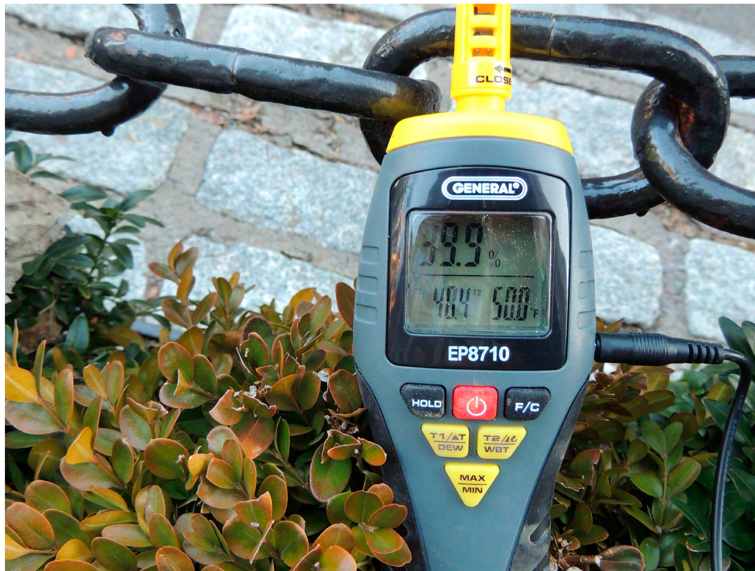
TEMPERATURE READING TAKEN IN NORTHERN-MOST TREE PIT, JANUARY 15, 2015. AIR TEMPERATURE: 40.4°, SOIL TEMPERATURE 50.0°
