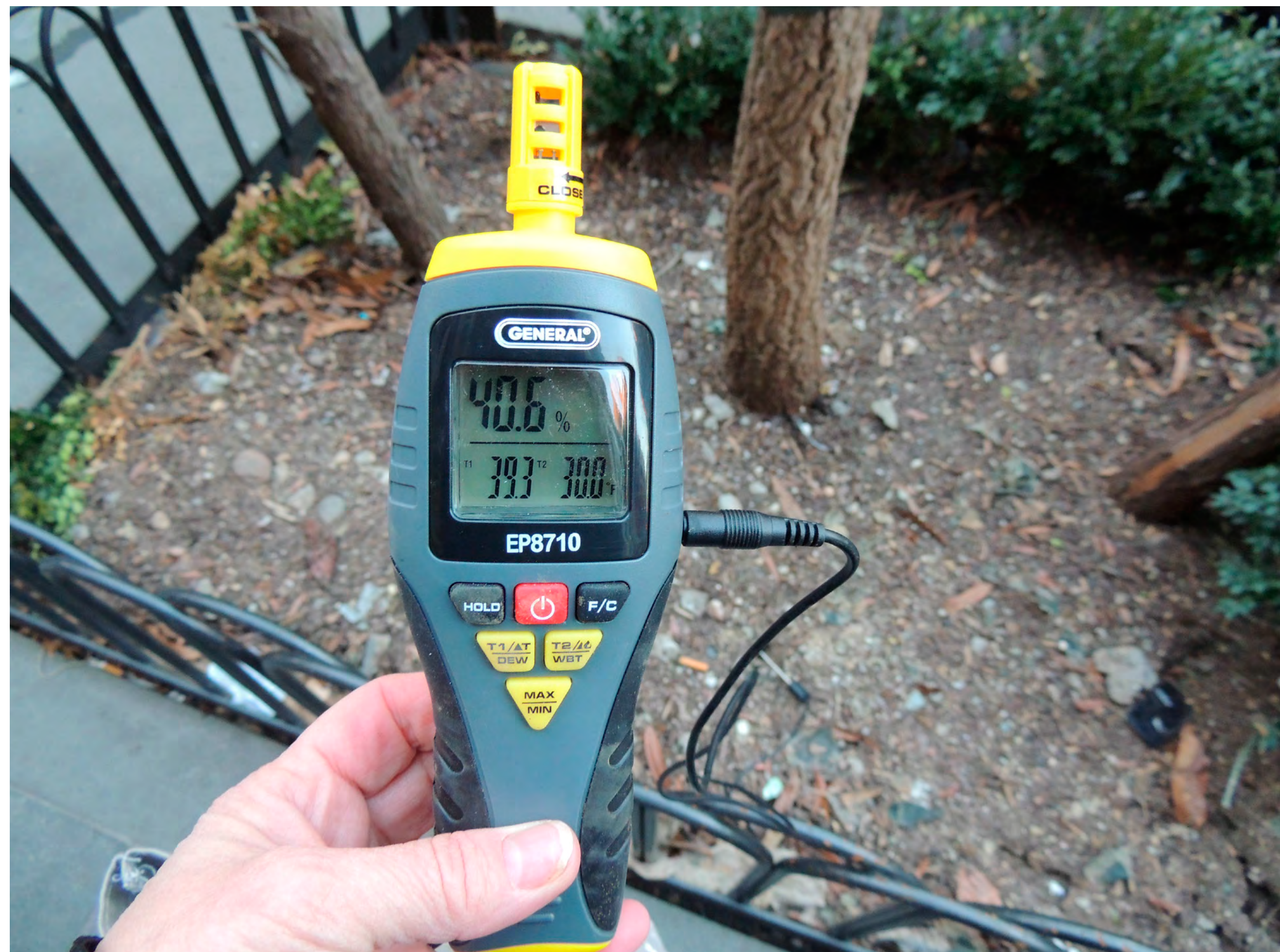
TEMPERATURE READING TAKEN IN TREE PIT ON GRAMERCY PARK SOUTH, JANUARY 15, 2015. AIR TEMPERATURE: 39.3°, SOIL TEMPERATURE 30.0° (SOIL WAS FROZEN)
