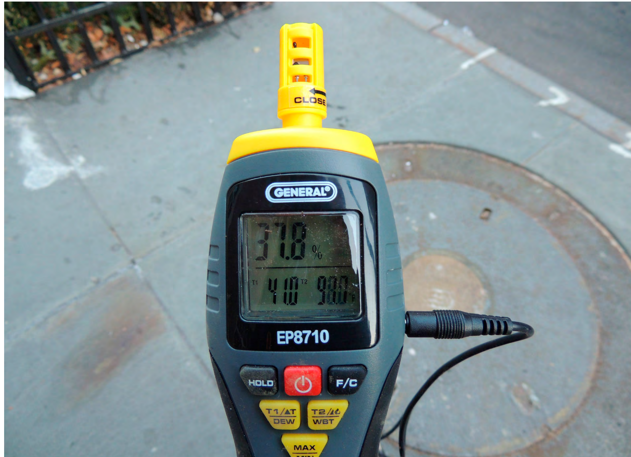
TEMPERATURE TAKEN AT CON-ED MANHOLE SURFACE TO SOUTH OF MIDDLE TREE PIT, JANUARY 15, 2015. AIR TEMPERATURE: 41.0°, MANHOLE TEMPERATURE 99.0°
