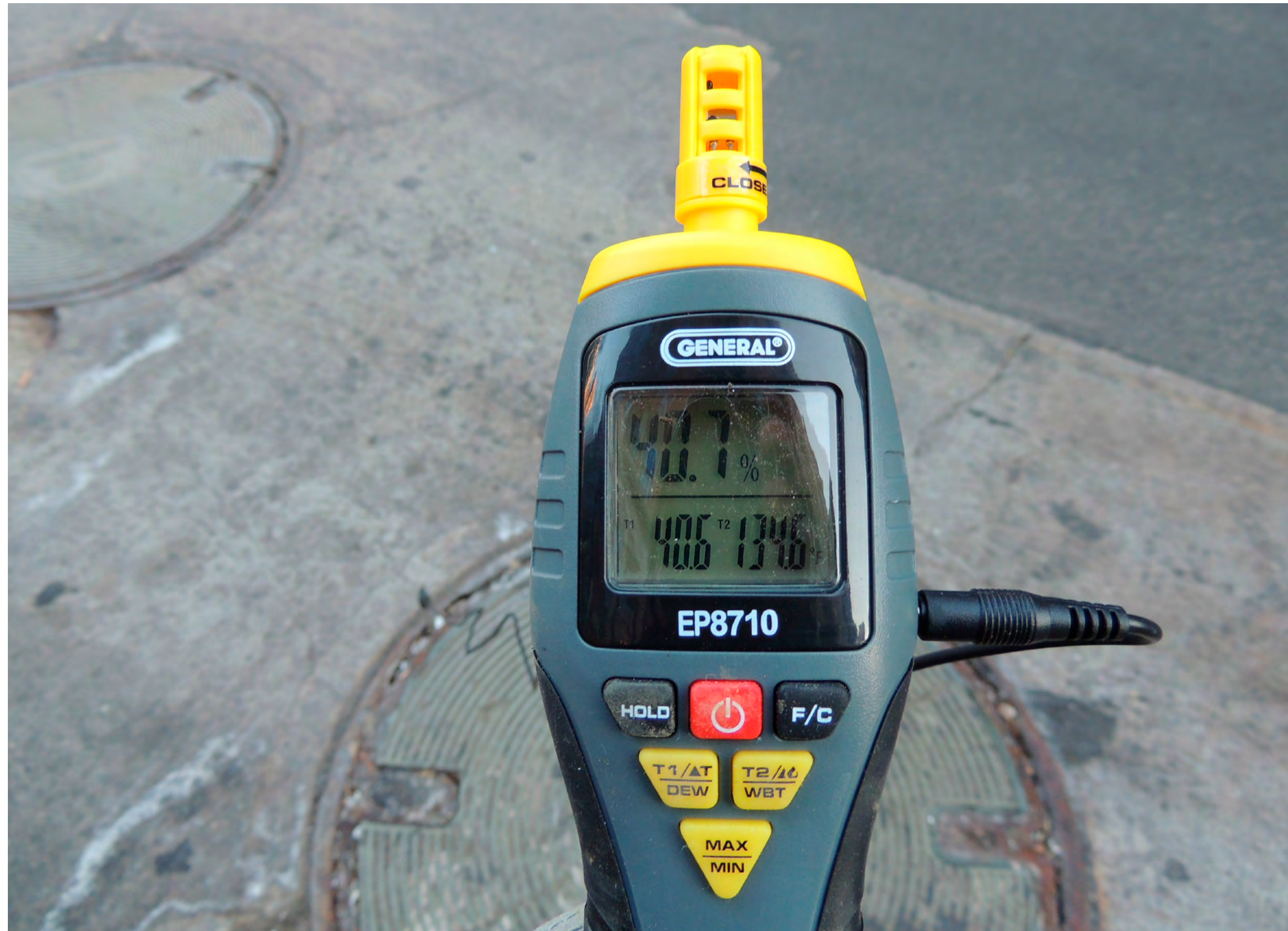
TEMPERATURE TAKEN AT CON-ED MANHOLE IN STREET TO EAST OF NORTHERN-MOST TREE PIT, JANUARY 15, 2015. AIR TEMPERATURE: 40.6°, MANHOLE COVER TEMPERATURE 134.6°
